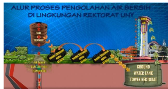
Water treatment at UNY
